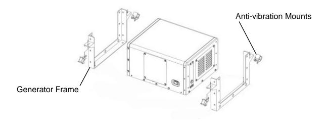
2.7 If using the slide out frame option, fix the anti-vibration mounting direct to the base of the generator then fix to the slide out frame.
